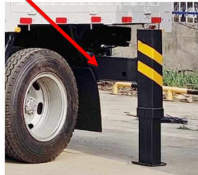
(Control Rear Hydraulic Legs)
