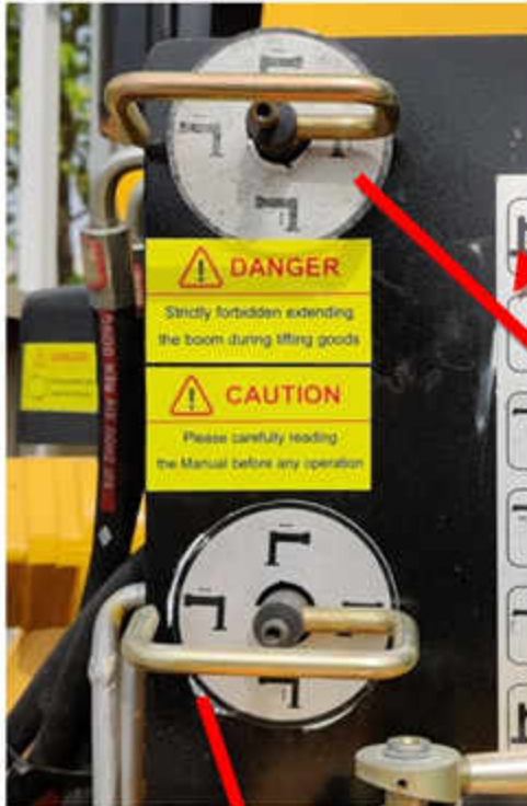
(Hydraulic legs control valves)
